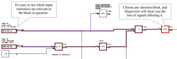
You can show the **output tree** for a block just as easily. As you trace signals onto other sheets, you can visually confirm that they are affected by the output of the original block of interest.
